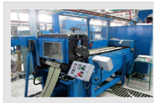
Continuous pasting production line
