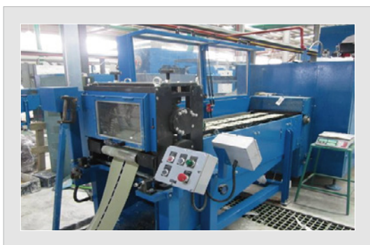
Continuous pasting production line
